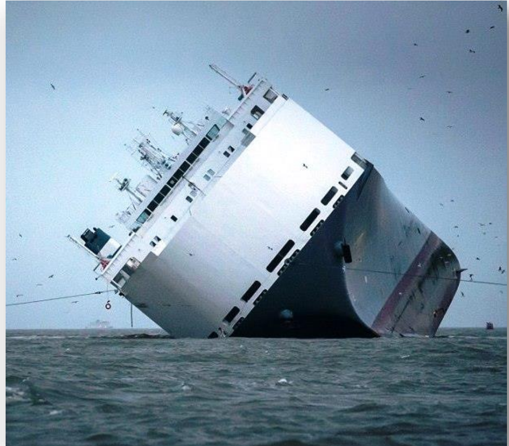
14- A bilging situation, causing free-surface effects.
