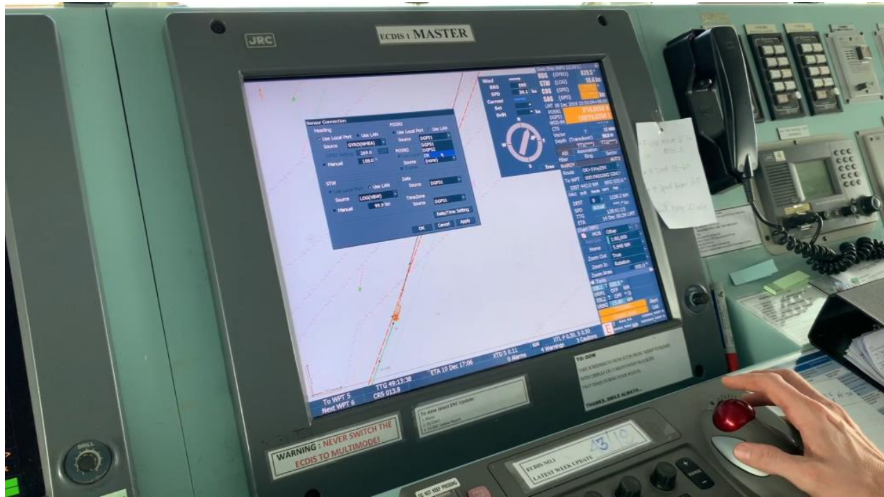
Figure 12. ECDIS sensor settings. Source: YouTube – Capt. Tymur
