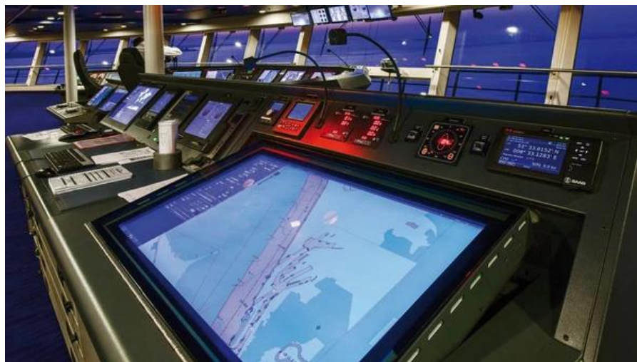
Figure 2. ECDIS device. Source: American Nautical Services.
