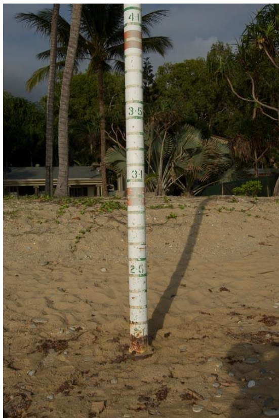
Figure 4. Tide pole gauge (Cali, 2012).
