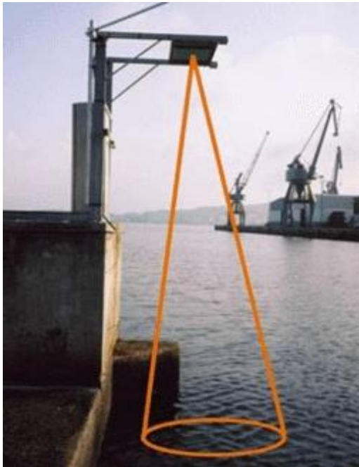
Figure 8. RADAR gauge (Turkey General Directorate of Mapping, 2020).
