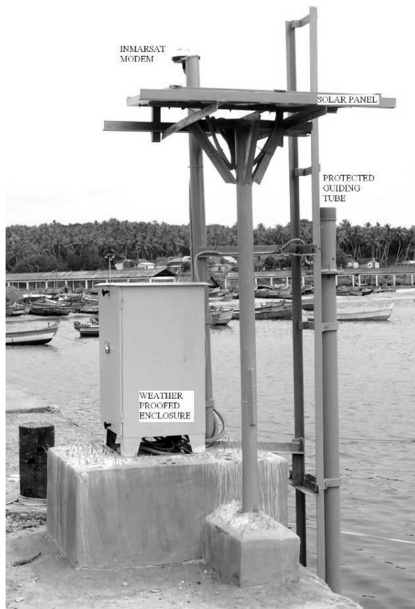
Figure 6. Acoustic tide gauge station (Zacharia et al., 2017).
